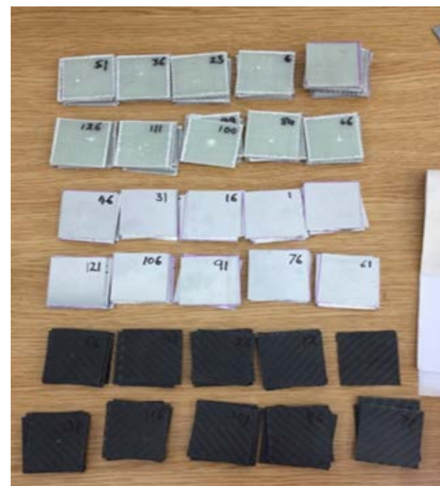
Images of all of the test samples, these include the damage and undamaged test samples.
