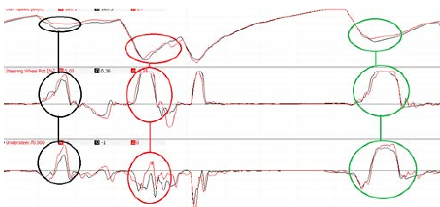
Figure 3 - Simulator test data with speed, understeer and steering percentage channels (Deion Atkinson, 2020)
