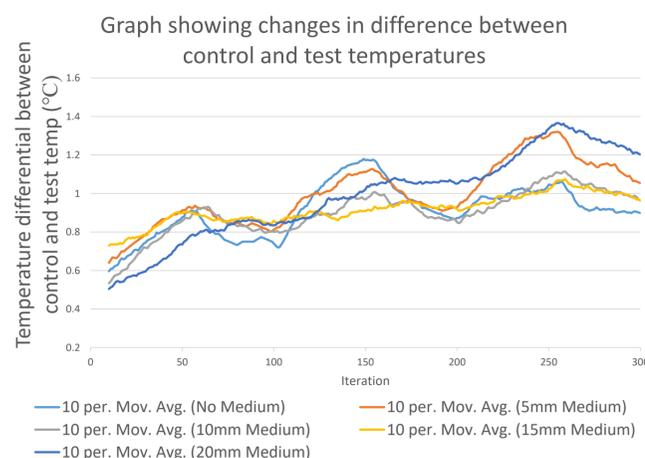
Figure 2 - Graph showing changes in difference between control and test temperatures for 5 varying mediums of simulated human tissue
