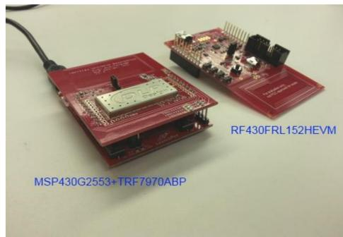
Figure 1 – Image of the development board and NFC plugin module (left) and development board for NFC based sensor (right) [2]
