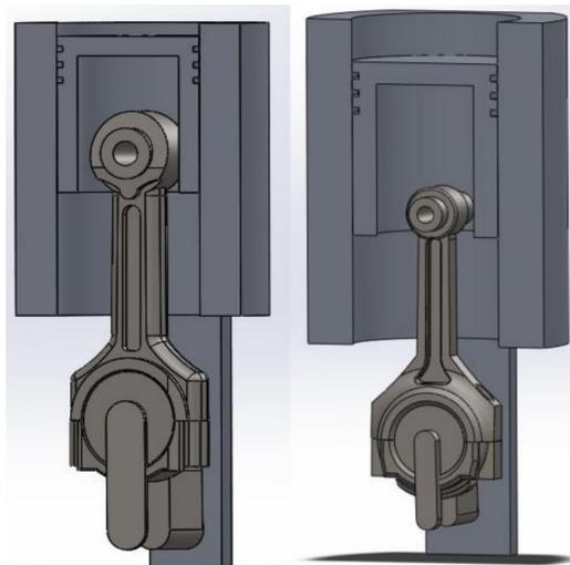
Figure 1. Cylinder Model Assemblies. Left: Ford Connecting Rod. Right: Triumph Connecting Rod.
