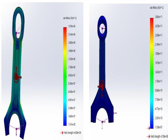
Figure 2 (Left). Ford Connecting Rod FEA Results, Von-misses
