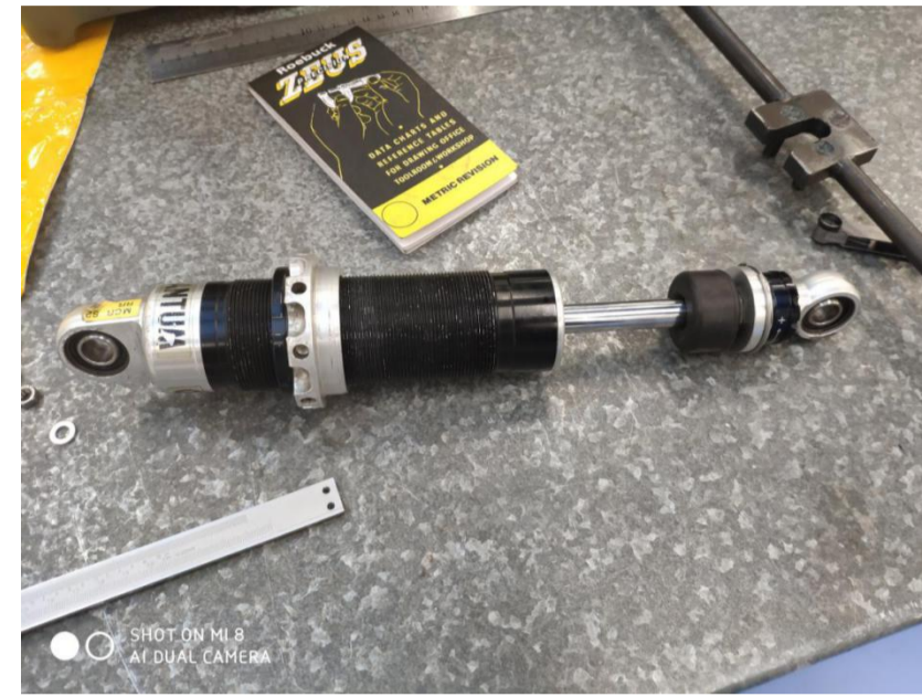
Figure 1. The mono-tube damper used in the experiments.
